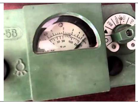
Measurement of exposure dose rate (radiation level) on the ground
