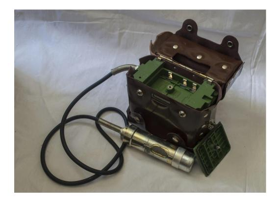
Radiometric control (ДП-5в)
