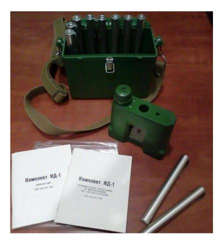
INDIVIDUAL DOSIMETER (ИД-1) Personal dosimetriccontrol device The purpose -to measure absorbed dose of gamma and neutron radiation (in the range from 0 to 500 rads) The unit of measure is red
